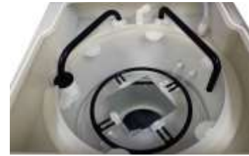
Example of Process Chamber with PTFE-Coated Stainless Steel Arms & Adjustable 4"x4" to 9"x9" SEMI Photomask Chuck
