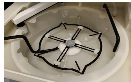
Example of Process Chamber with PTFE-Coated Stainless-Steel Arms & Adjustable 4"x4" to 14"x14" SEMI Photomask Chuck
